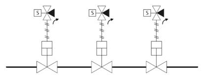
In many cases it is impracticable to install three valves in series. Non-compliance is widespread. The most common practice is to use only two valves in series, either in a double block or a double block and bleed arrangement.
