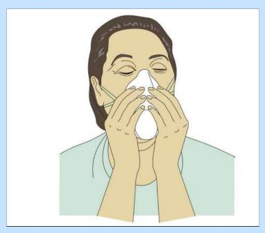
If the respirator has an exhalation valve, cover the filter surface with your hands as much as possible, then inhale. The seal is considered satisfactorily if the face-mask collapses on your face and you don't feel air passing between your face and the face-mask.
