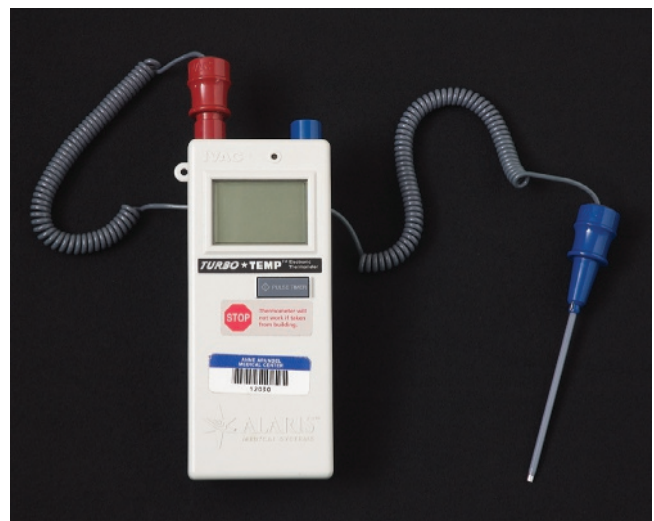
Figure 20-5 A battery-operated electronic thermometer.
