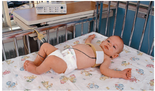
FIGURE 40.14 The home apnea monitor uses a soft belt with a Velcro attachment to hold two leads in the appropriate position on the chest.
